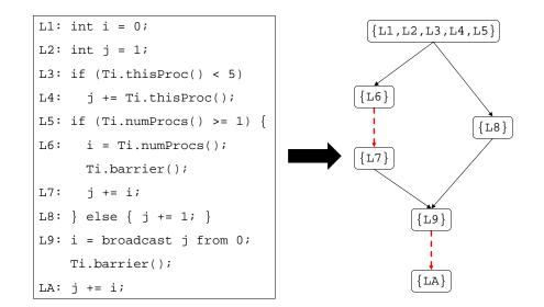
Figure 2: The graph of code segments for an example program. Each node in the graph corresponds to a segment, and the dashed edges correspond to barriers.
